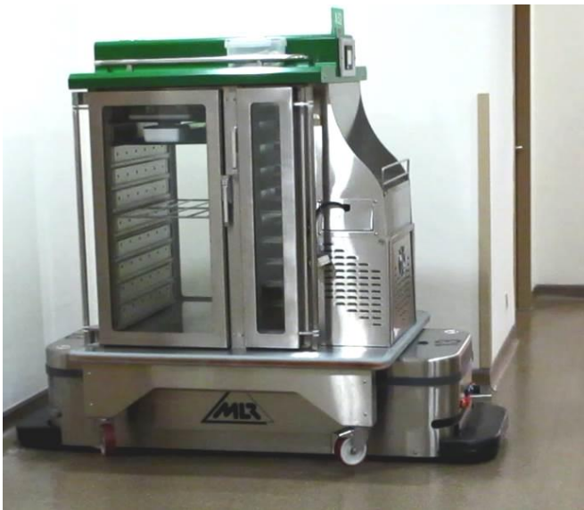
Figure15: Typical AGV with a supply trolley
